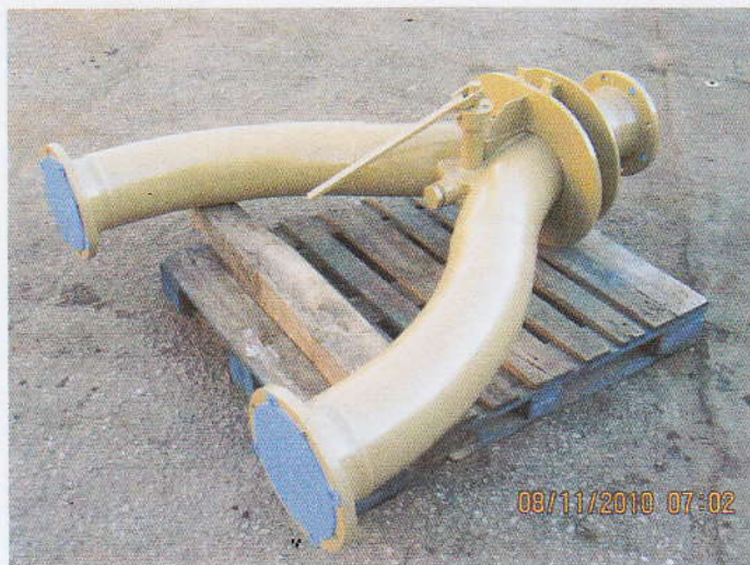
Picture below shows one of two 8-inch ANSI 150 Non-sealing Pig Switches with 5 diameter bends.
